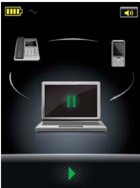
Figure 59: The current (active) call is put on hold; no other calls are waiting
