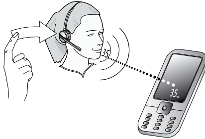
Figure 40: To use voice-activated dialing, tap the multifunction button and speak the appropriate voice tag
