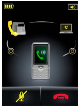
Figure 87: The merged calls are put on audio-hold when the new call is accepted.
