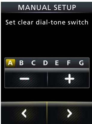
Figure 16: Manual clear dial-tone switch position selection for Jabra PRO 9465 Duo / Jabra PRO 9470
