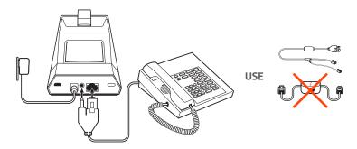
**IMPORTANT** Use configuration **A** on the bottom of the base, which works for most phones including Cisco phones.
