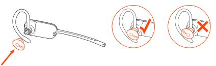
**NOTE** Ensure the large end of the eartip points to the microphone.
