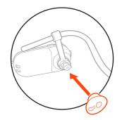
**NOTE** Ensure the large end of the eartip points to the microphone.
