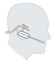
4 With a finger on the headset indicator light, push in until the microphone rests as close to your cheek as possible without touching.
