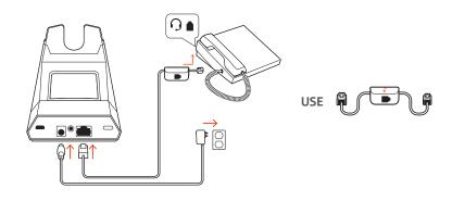
• Connect one end of the telephone interface cable to the back of the base
