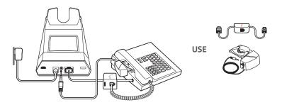
**IMPORTANT** Cisco phones use configuration  ${\bf D}$  on the bottom of the base. Most other phones use default configuration  ${\bf A}$ .
